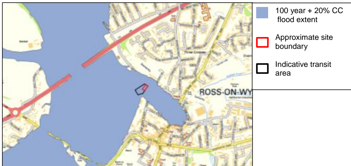
Figure 5 EA's River Wye hydraulic model flood extent for the 1% annual probability event plus 20% climate change scenario
