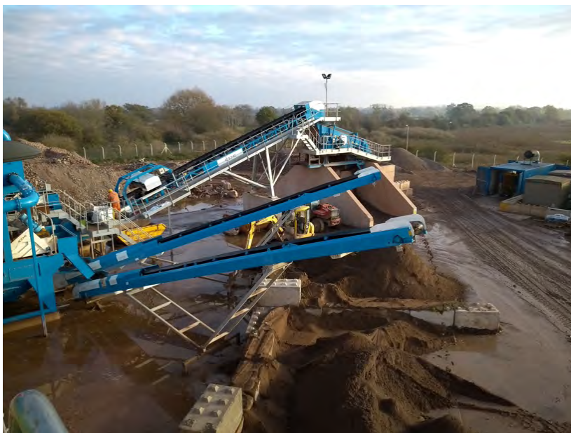
Photograph M02_1: Construction, demolition and excavation waste recovery plant
