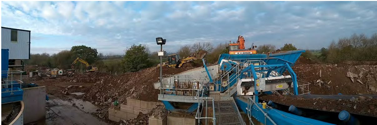
Photograph W13_1: Recycling/recovery plant, waste being tipped into hopper
