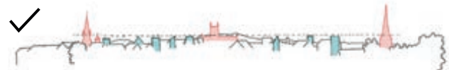
Careful consideration of how new roofs nestle into the varied roofscape, below the line of the nave of the Cathedral
