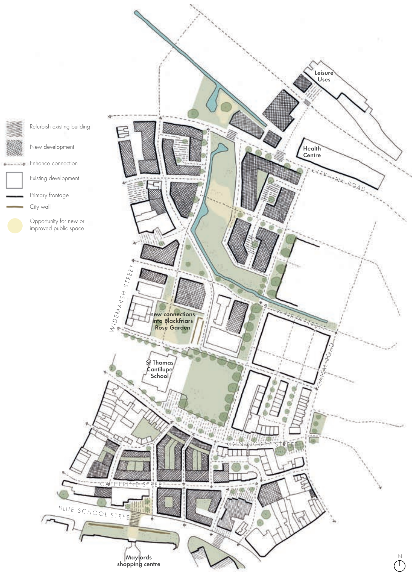
Figure 1.73: An indicative sketch illustrates how a new green route from the city centre to the City Link Road and new health centre could be delivered
