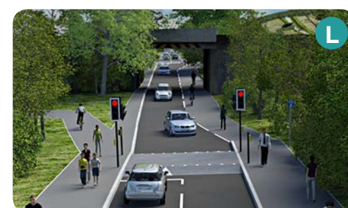
Signalised one way working over/under railway bridge
