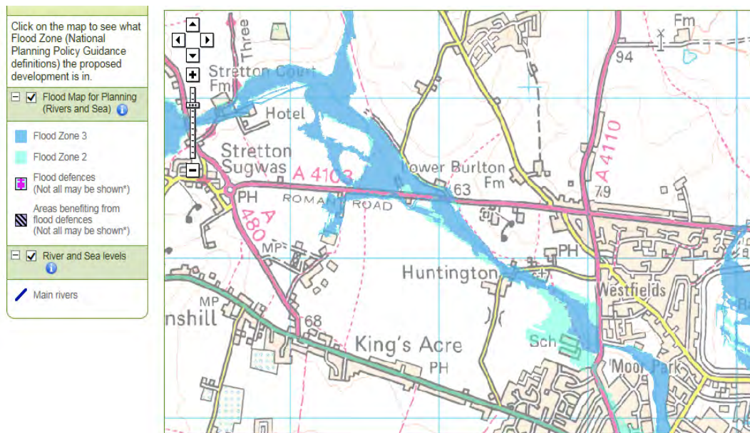
Fig 6.2 Extract From Environment Agency's Flood Risk Map to Show Flood Zones at Proposed Three Elms Strategic Location.
