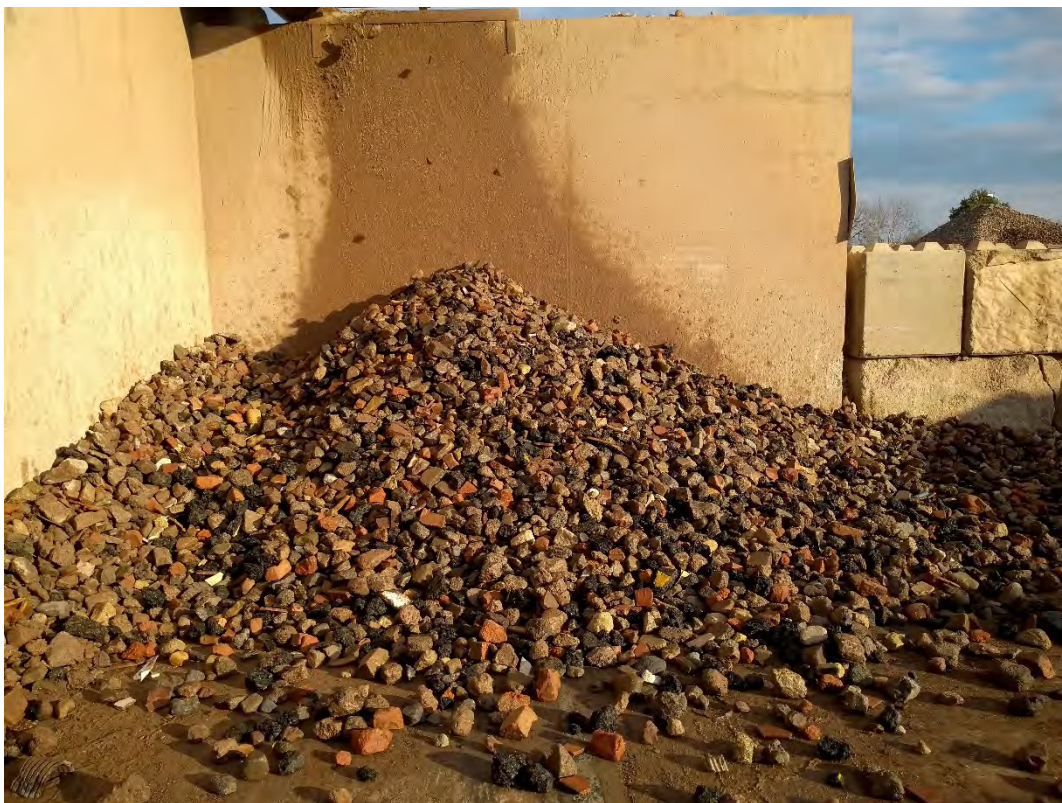
Photograph W13_4: Recovered aggregate
