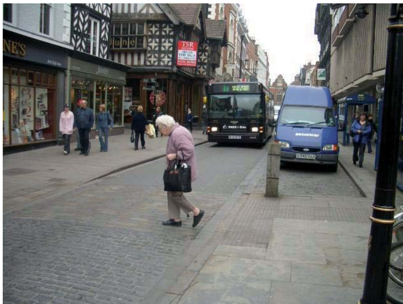
In Shrewsbury, narrow carriageways, courtesy crossings and sensitively marked parking bays help to create a slow speed environment
