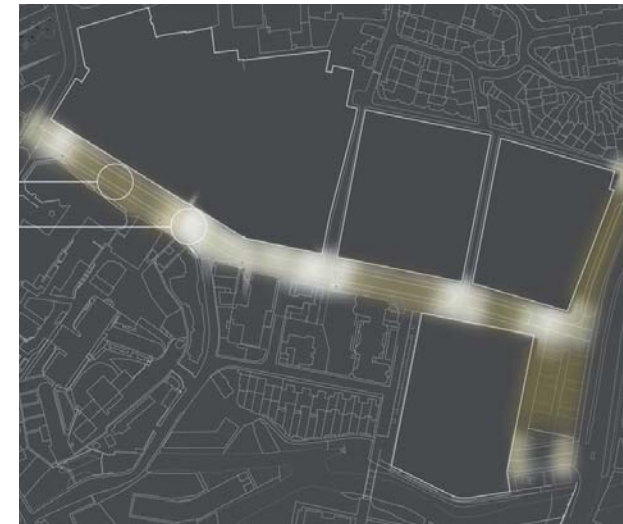
Illumination plan for Oxford Westgate illustrating the principle of highlighting spaces and intersections
