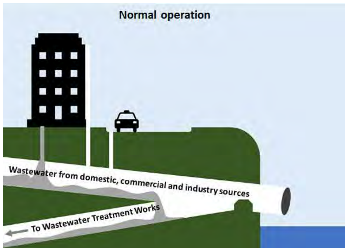
Figure 6-2 Storm overflow operation in normal conditions
