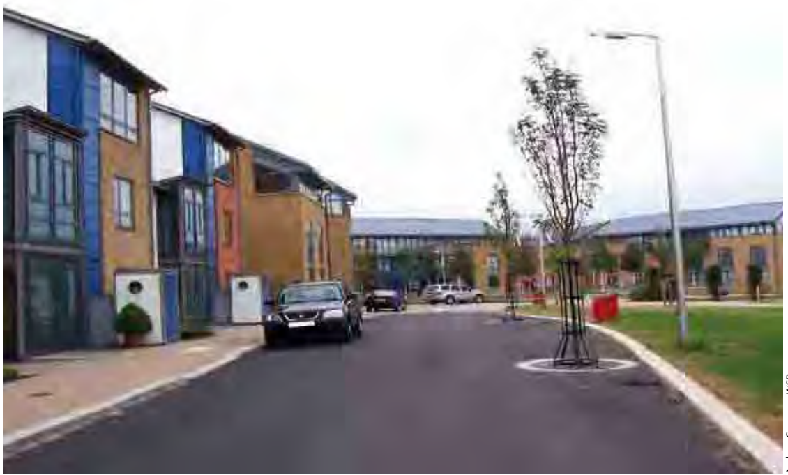
Figure 7.15 Trees planted in the highway at Newhall, Harlow, help to reduce vehicle speeds.
