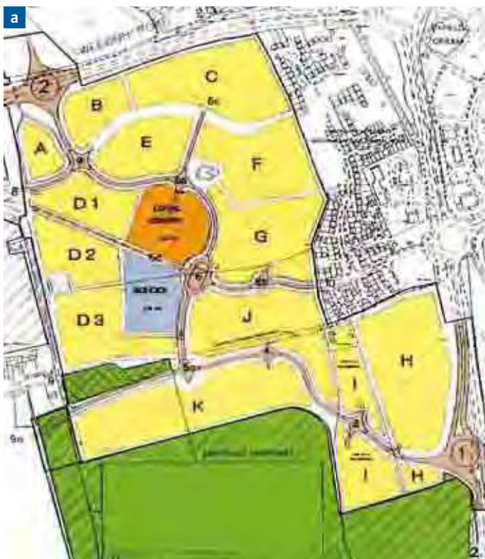
Figure 4.11 Alternative proposals for a development: (a) is highways-led; while (b) is more attuned to pedestrian activity and a sense of place.
