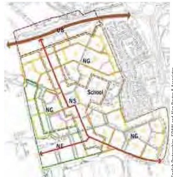
Figure 3.9 Street network diagram for Upton, Northamptonshire, showing the main route through a connected layout and linkages to key spaces and places within the development, with street character types identified.
